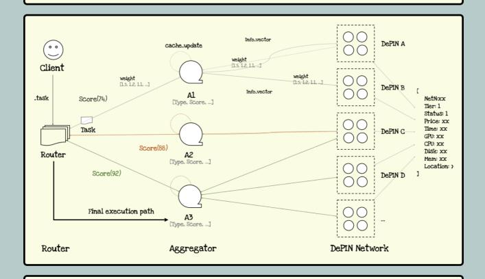
Dynamic routing is considered in complex scenarios, where a task needs to be split into multiple subtasks, and it requires dynamically finding the optimal combination across different DePIN networks. Here, we provide 3 strategies based on the client's cases:
