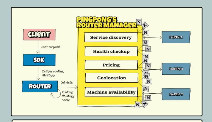
The PINGPONG router manager actively gets data from the underlying DePIN networks and keeps a record for service discovery, health checkups, pricing, machine distribution status, and machine availability.
